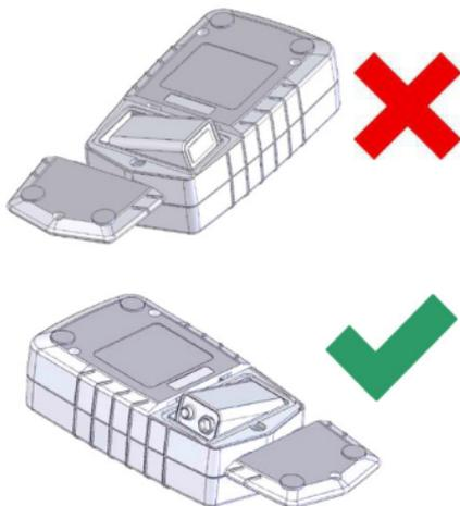
**IMPORTANT** - When replacing the battery ensure the bottom of the 9V battery is inserted first as shown above. Improper battery insertion may result a loose battery and poor battery connection.
