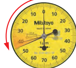
Indicator trackability depends on maintaining gear-train stability
