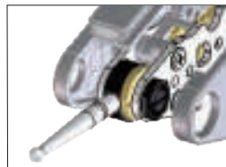
Stylus bearing screw held in sub-plate.
