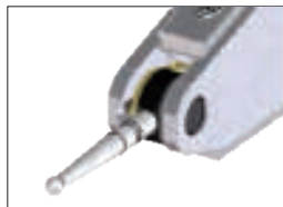
Stylus bearing screw held in frame.
